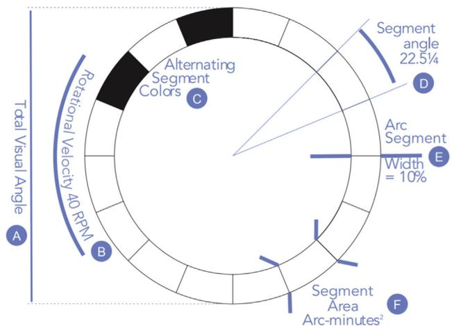
**FIG 1.** Fundamental geometry of the dynamic optotype (Dyop): total circular diameter or visual angle (A), speed of rotation (B), color contrast (in this study black and white) (C), segment angle (D), segment arc width (E), and area of each segment in arcmin<sup>2</sup> (F).
